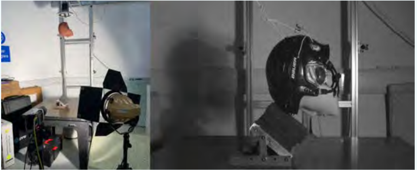
Testing hockey helmets for protection against concussive impacts
